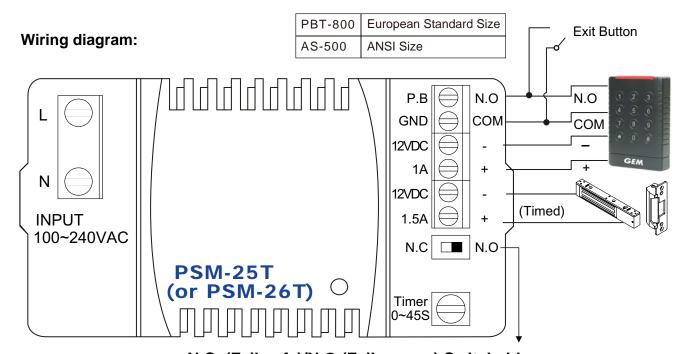
N.C. (Fail-safe)/N.O.(Fail-secure) Switchable
